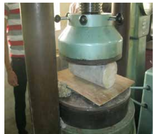
Fig 3 Tensile strength of the specimen before repair
