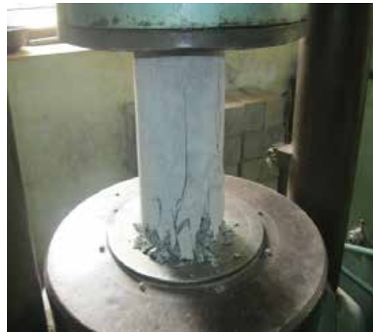
Fig 2 Compression strength of the specimen before repair
