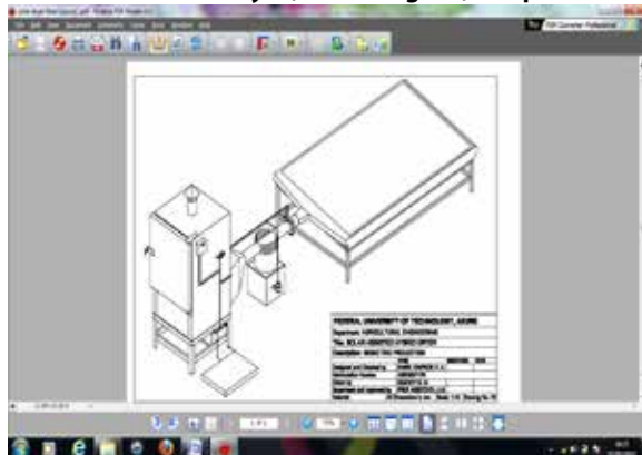
Figure 1: Isomeric veiw of a solar assisted hybrid dryer
