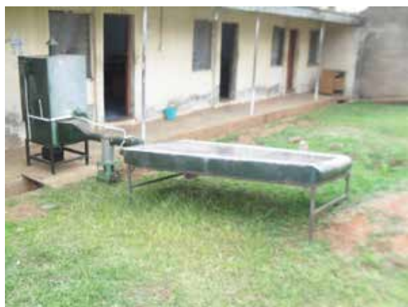
Figure 3: Pictorial View of Hybrid Dryer
