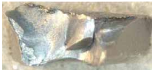
Figure 4- Gear Chip( 4 mm x 2 mm )
