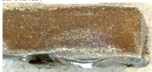
Figure 2- Gear Chip( 5 mm x 2 mm )
