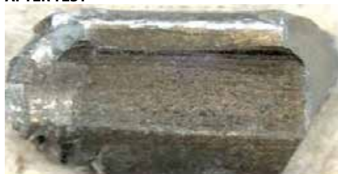
Figure 7- Gear Chip( 4 mm x 4 mm )
