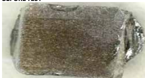
Figure 6- Gear Chip( 4 mm x 4 mm )
