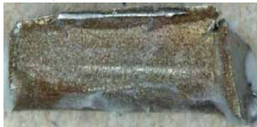
Figure 3- Gear Chip(5mm x 2mm )
