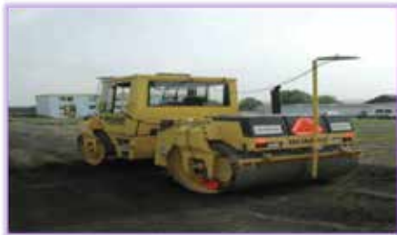
Fig.1. OSYRIS project sensor-based compactor
