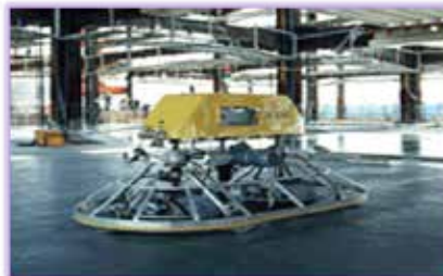
Fig.5. Takenaka's concrete compactor robot
