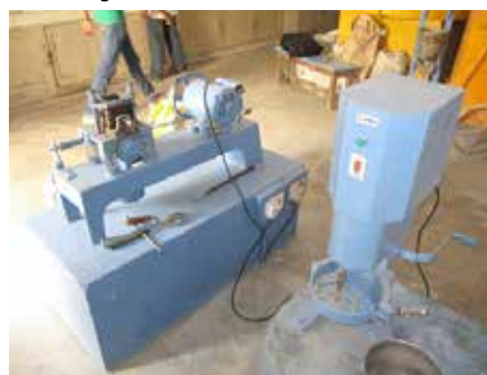
Fig 3: Set up of Vibrating Machine and Crucible for Mixing Cement and Fine Aggregate (Sand)
