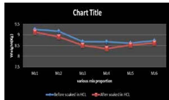
Fig 4: Change in Mass of the Cubes Soaked in HCL for M30 Grade Concrete
