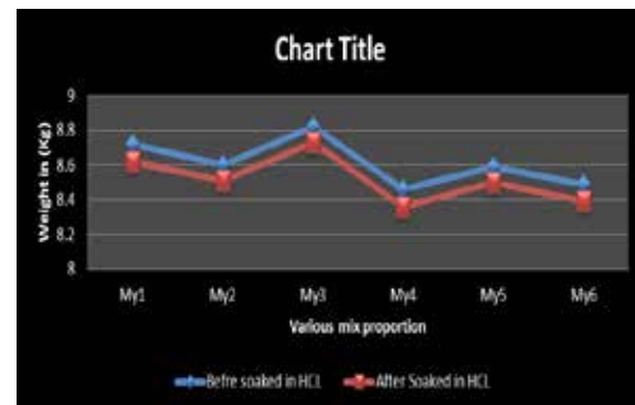
Fig 3: Change in Mass of the Cubes Soaked in HCL for M25 Grade Concrete
