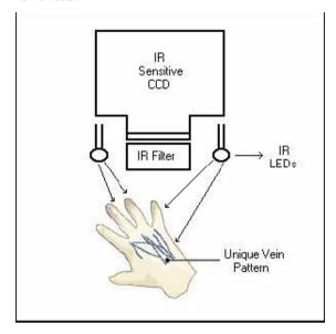
Whereas Mohamed Shahin, Ahmed Badawi, and Mohamed Kamel proposed [5], biometric authentication using hand vein patterns, they designed a system a near IR cold source to provide back-of-hand illumination. The IR cold source is a solid-state array of 24 LEDs (light emitting diodes). The diodes are mounted in a square shape, 6
