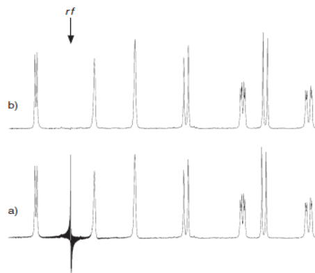
Figure-2 The aesthetically unappealing decoupler frequency 'spike' sometimes observed in homonuclear decoupling experiments as in (a) can be readily removed by setting the transmitter and decoupler frequencies to be the same, as in (b).
