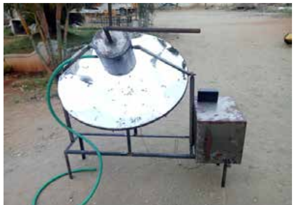
Figure:1 Solar water purification by using thermal method.
