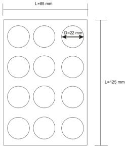
Fig. 2.Shape and dimensions of twelve multiwell plate
