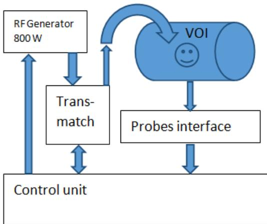
Figure 1. The design of the system
