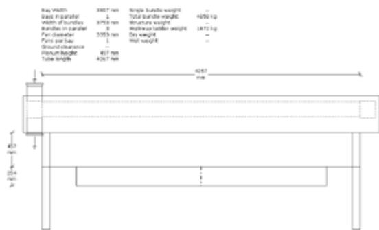
2-D view of Air cooled heat exchanger<sup>[6]</sup>
