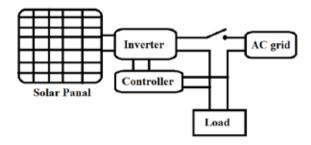
Figure1 Power Generation structure of Grid connected Photovoltaic System
