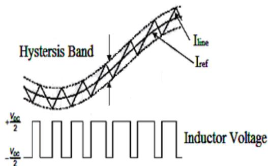
**Figure5 Controlling action of Hysteresis control Method**
