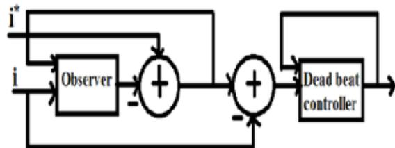
**Figure3 Basic Block Diagram of Dead-Beat Control**
