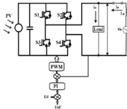
Figure2 Basic Structure of Voltage Source Inverter
