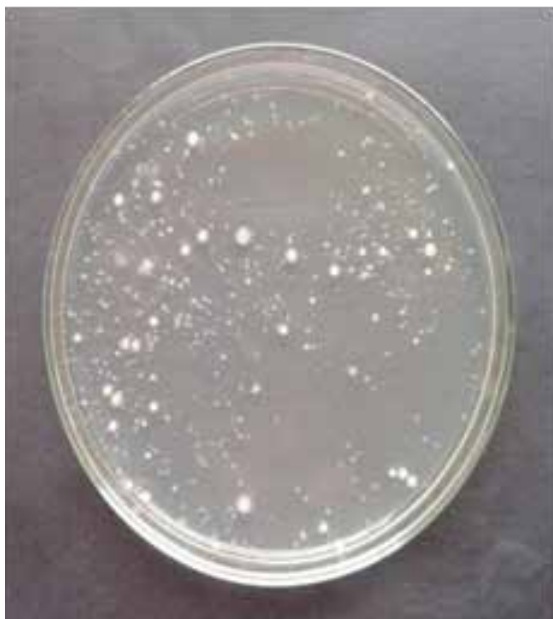
Fig.3 treated water with seed powder 100mg/l showing lesser no. of microbial colonies than fig.1 and 2
