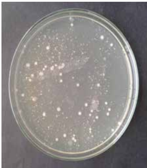
Fig.2 treated water with seed powder 50mg/l showing less no. of microbial colonies than fig.1
