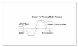
As shown, across the width, the accumulated solids can be removed every fifteen days and taken to MSW landfill sites. The screen with a gabion wall will allow water to flow through but will capture all floating matter.
