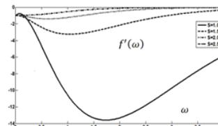
Figure 2: Velocity profiles with  $Da = 1$
