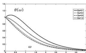
Figure 6: Temperature profiles with  $S = 2$  and  $P = 0.71$
