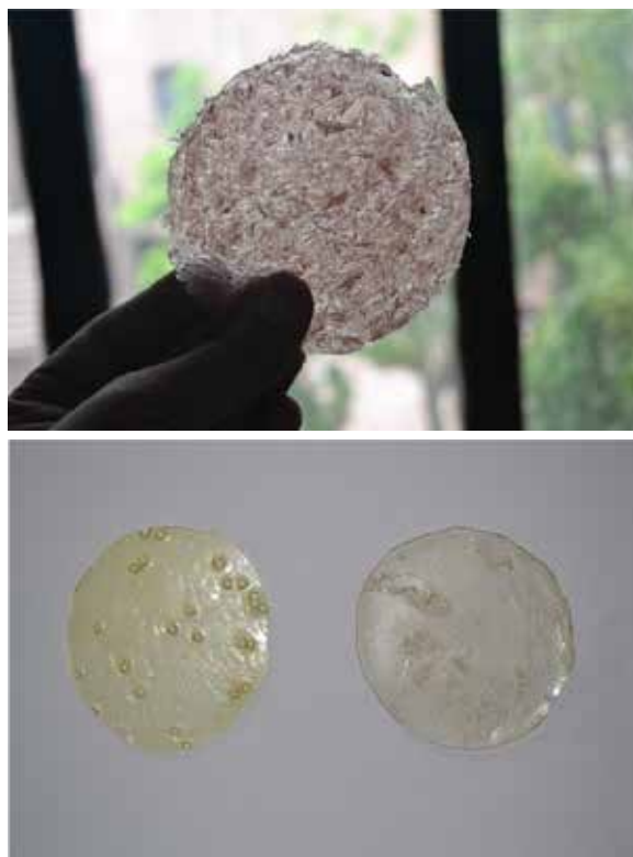
Fig. 2 Photograph of (a) sisal fibre reinforced castor oil derived polymer composite (b) polymer synthesis using Acetone (left) and MEK (right) as solvent
