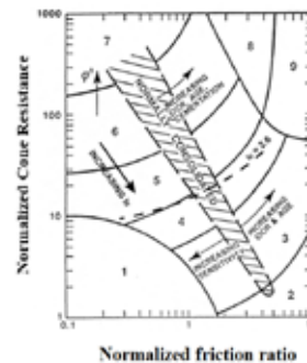
Fig 1. Soil Behaviour Chart
