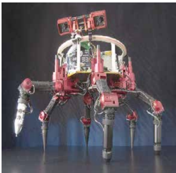
FIGURE 4: A new class of multi-limbed robots called LEMUR (Limbed Excursion Mobile Utility Robot) is under development at JPL
