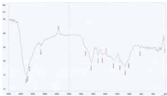
Figure 5 FTIR for NaOH treated coconut fiber
