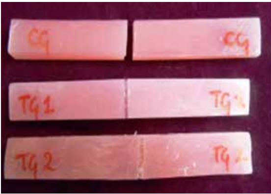
Figure 6: Broken specimens ( CG: Control Group, TG1: Test Group 1, TG2: Test Group 2)
