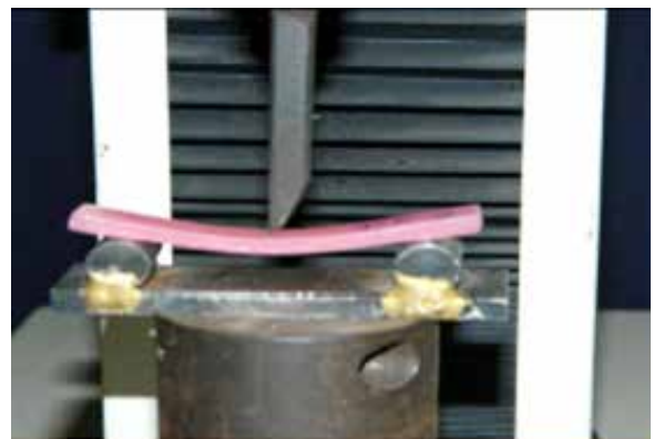
Figure 5: Flexion of test specimen during testing
