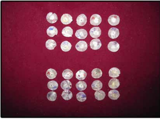
FIG 3: SECTION GROUP A ( GLASS FIBRE POST ) SPECIMENS
