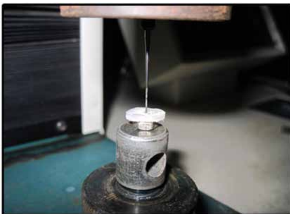
FIG 5: SECTION PLACED ON THE UNIVERSAL TESTING MACHINE FOR 'PUSH OUT TEST'
