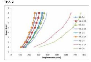
From the results it has been observed that with which the increase in vierendeel panel width deflections displacement increases, but the storey shear, bending moment and axial force also increases slightly.
