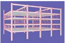
Figure 1: Typical 3-D model of standard staggered trusses supporting hollow core slabs
