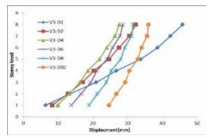
V refer to vierendeel width and D refers to the number of diagonal truss chords on one side
