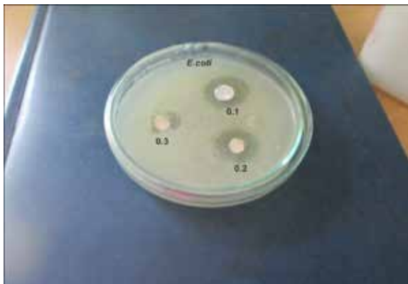
Figure 3: Antibacterial activity of disc for different concentration of Zinc oxide Nanopowder (Escherichia coli).
