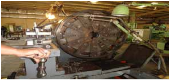
Figure 3 rough machining of seal ring on lathe machine Procedure:-
