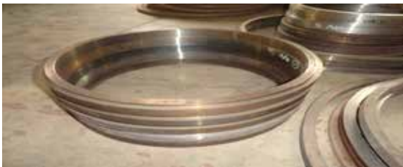
Figure 4 rough machining of seal ring completed
