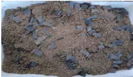
Fig 4. shredded rubber tire mixed with black cotton soil
