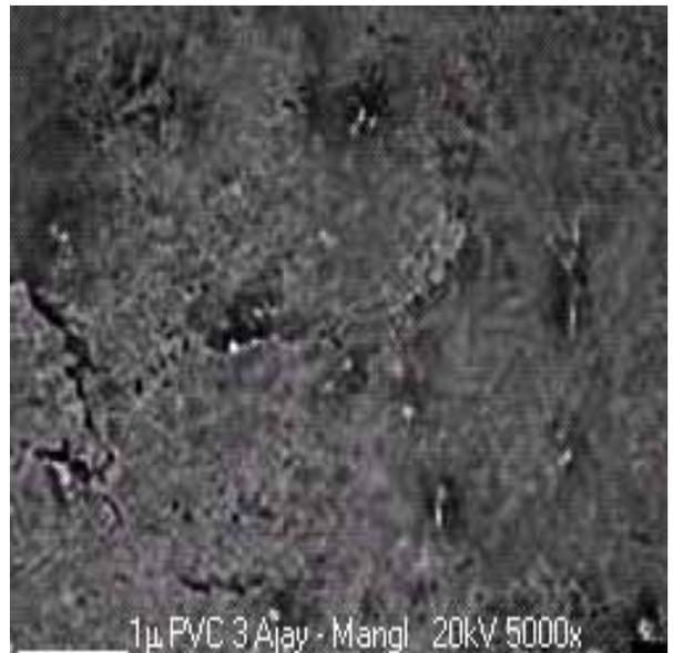
**Figure 7: SEM Photograph of 70% PVC 30% CCTO Composite**
