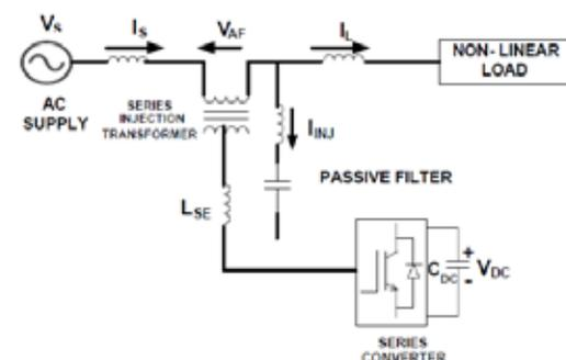
Fig . Line diagram of hybrid active filter
