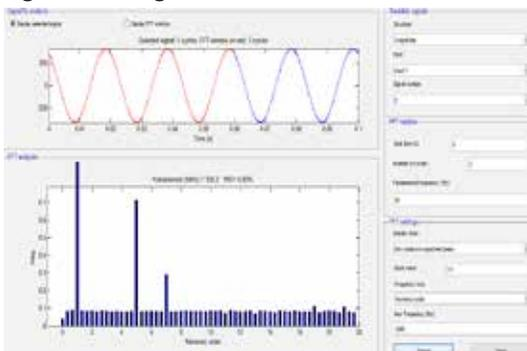
Fig. Load Voltage with %THD for Phase C
