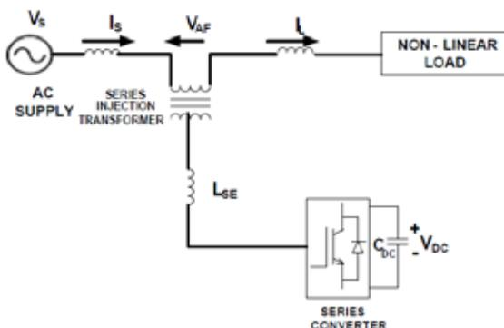
Fig . Line diagram of series active filter
