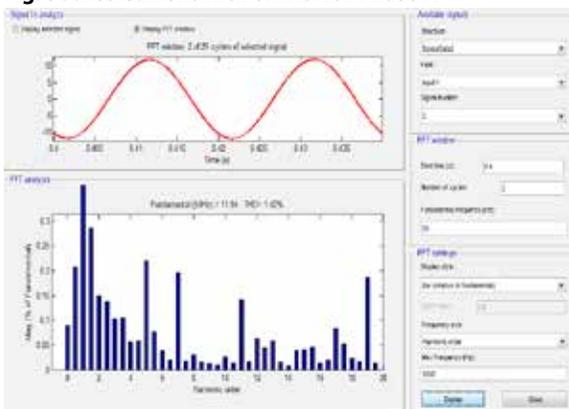
**Fig. Source Current with %THD for Phase B**
