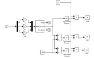
Fig. Simulink model of control scheme for series APF
