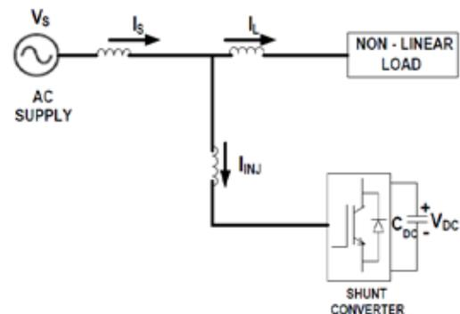
Fig . Line diagram of shunt active filter
