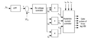
Fig. Control Scheme of UVTG in Shunt APF
