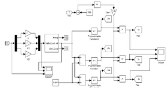
Fig. Simulink model of control scheme for shunt APF
