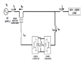
Figure 2.9 Line diagram of unified power quality conditioner
