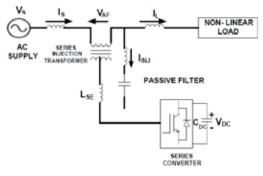
Fig . Line diagram of hybrid active filter
