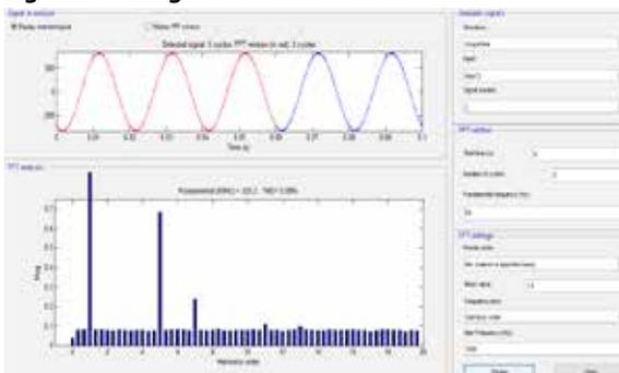
Fig. Load Voltage with %THD for Phase B
