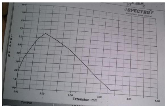
**Fig 6.Strength of welded specimen by using mild and stainless steel filler material**
