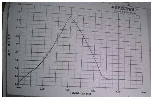
**Fig 5.Strength of welded specimen by using mild steel filler material**
