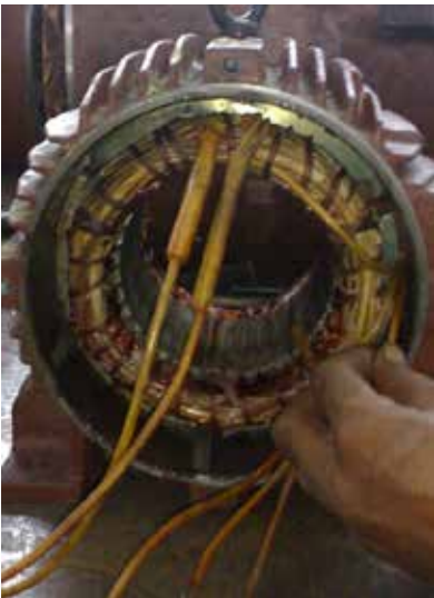
Photograph 2. Six phase stator after winding
