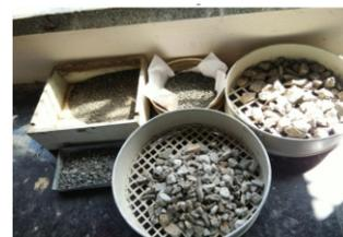
Figure 2: Sieve Analysis of Aggregates
