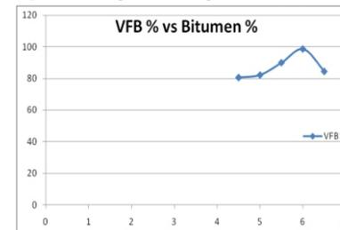
Figure 8: Graph showing Voids filled with Bitumen(VFB) vs Bitumen %
