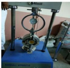
Figure 1: Marshall Apparatus
