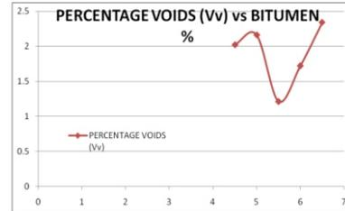
Figure 7: Graph showing Percentage Voids(Vv) vs Bitumen %
