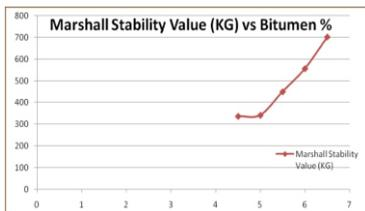
Figure 4: Graph showing Stability vs Bitumen %
