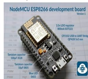
Fig 1: ESP8266-12E board Description
