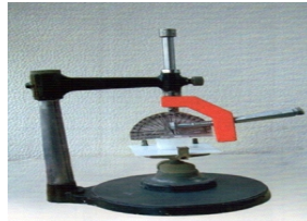
Fig.2: Modified Ney surveyor used in the Polymerizing resin study for preparing the embedded teeth
