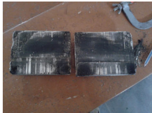
Fig. 2: Section showing honeycomb structure
