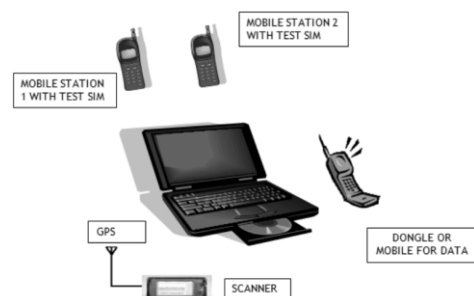
Figure 1. Equipments set up for Drive test
