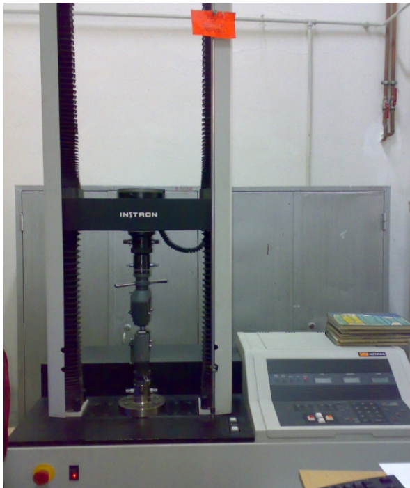
Fig. 4.a. The traction, compression and buckling testing machine Instron 4303.
