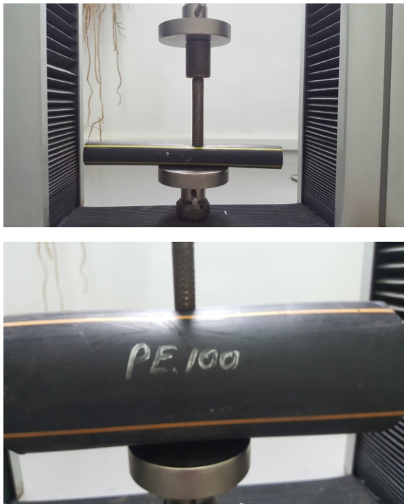
Fig. 5. Imprinting the polyethylene pipes with a 1000 N force in order to measure the deformations produced by the four pins
