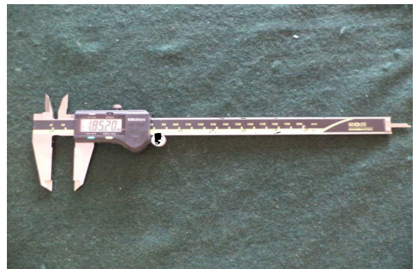
Fig. 3: Digital Vernier Callipers
