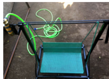
Figure 2: Water Lifting System Final Assembly
