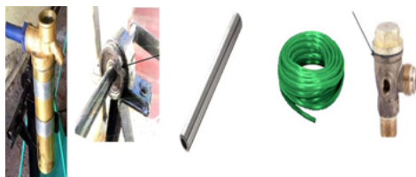
Figure 1: Components of water lifting system. Left to Right (Reciprocating Water Pump, Pedestal Bearing with C Type Clamp, Shaft, PVC Pipe and Non Return Valve for Water Suction)
