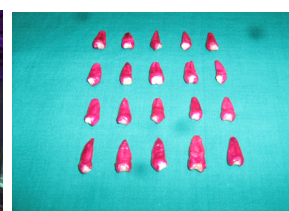
SPECIMENS AFTER COATING WITH NAIL POLISH Fig 6
