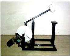
Fig 3: Prototype Automatic Hammering Machine
