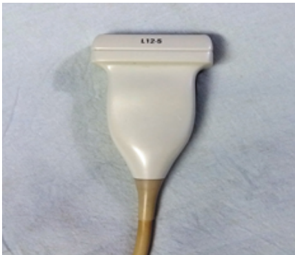
Figure 4: Shows ultrasound transducer used is Broadband Linear Array Transducer 5 to 12 MHz extended operating frequency range. (Philips medical system)
