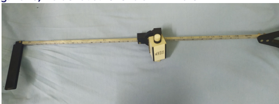
Fig. no 10) Holder at other end of RAF Rule
