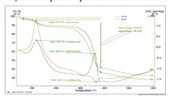
Figure 7) STA analysis of layer 1a and 2a of cardboard box after treatment
