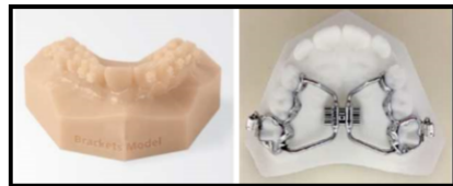
Dental model and Rapid Palatal Expansion model 3D printed from a STL generated file
