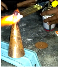
Fig.2. brazing process attaching copper tube
