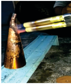
Fig.1 brazing process for diffuser
