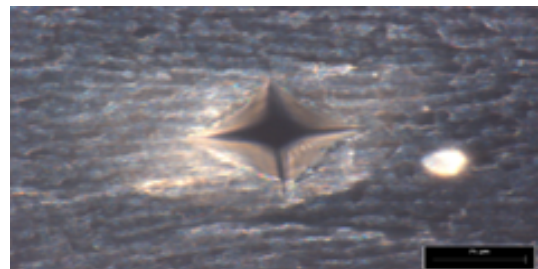
Figure 2. Optical microscopy photography of the indentation produced by the enamel microdurometer, (sample2.4), magnification 100x, scale 25mm under a load of 300 g for 15 seconds.
