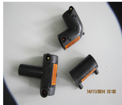
Figure 11: Elements used in assembling the polyethylene pipes
