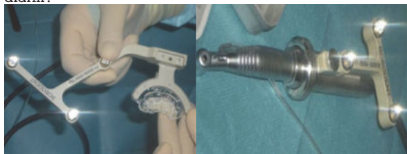
Fig. 9, 10 : Robodont: radiological guide and the extremity of drill present optical marks to give the spatial position
