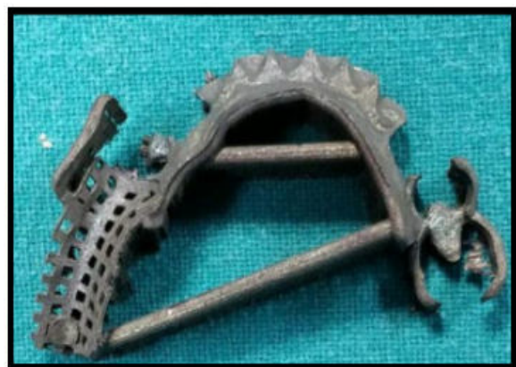
Fig.4- Framework After Laser Sintering Of Cobalt Chrome Alloy Powder
