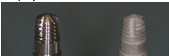
Fig. 9. The machined and nano etched implant surface
