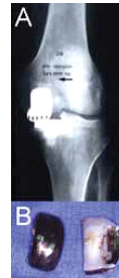
Fig.3 Wrong Component sizing or positioning may lead to edge loading (A) resulting in increased wear and implant failure (B).
